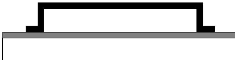
When the BPSG is removed, the fixed-fixed beam is held to the nitride by its conformal supports in the region where the BPSG holes were created. The section of the beam in the middle is now free to deflect when an external force, such as a pressure or electrostatic load, is applied.
